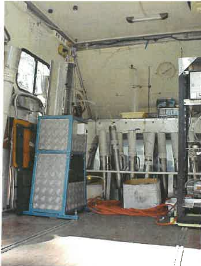
Figure 2.2 - Interior view of CSIRO mobile gas testing laboratory showing the fast desorption crusher.
