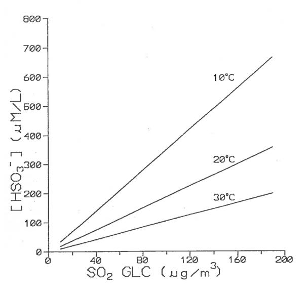
Figure 13 Calculations of the equilibrium concentrations of HSO<sub>3</sub> in rain water as a function of SO<sub>2</sub> concentration and for different ambient temperatures.
