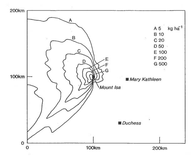
Figure 12 Isopleths of annual average dry deposition of SO<sub>2</sub> for the four year average and 300 k tonne emissions.
