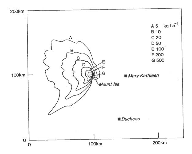
Figure 11 Isopleths of annual average dry deposition of SO<sub>2</sub> for the four year average and for base case emissions.
