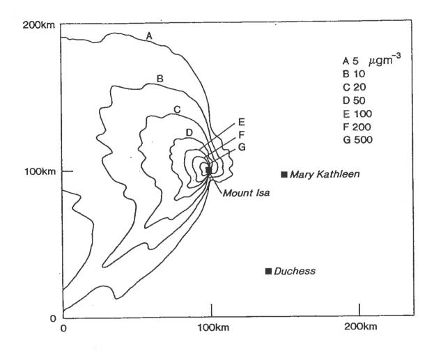
Figure 10 Isopleths of annual average ground level concentration of SO<sub>2</sub> using the four years of wind data assuming 300 K tonne emissions.
