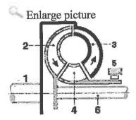
Hydrodynamic converter 1 Power, 2 Turbine, 3 Pump, 4 Stator, 5 One-way clutch, 6 Output.
