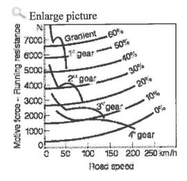
Running diagram for car with automatic transmission and hydrodynamic trilok converter under full throttle
