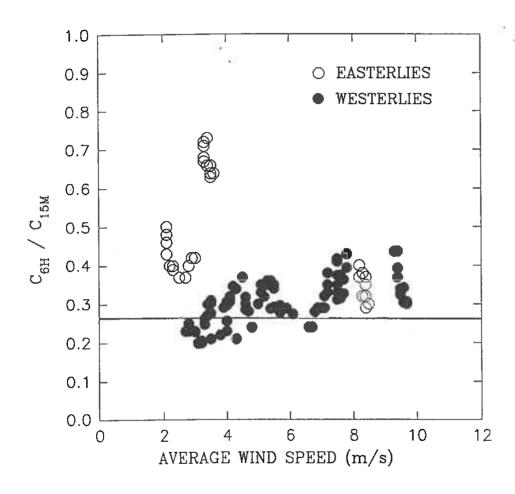
Figure 3 Ratio of 6 hour peak glc to average 15min peak glc as a function of wind speed (line represents n=0.41).
