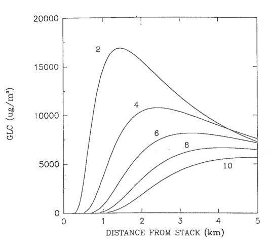
Figure 4 Centreline glc as a function of distance from stack for windspeeds 2,4,6,8, & 10m/s - Enhanced copper smelter emissions.
