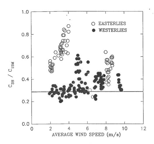
Figure 2 Ratio of 3 hour peak glc to average 15min peak glc as a function of wind speed (line represents n=0.5).
