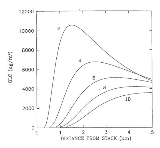
Figure 5 Centreline glc as a function of distance from stack for windspeeds 2,4,6,8, & 10m/s - Base case copper smelter emissions
