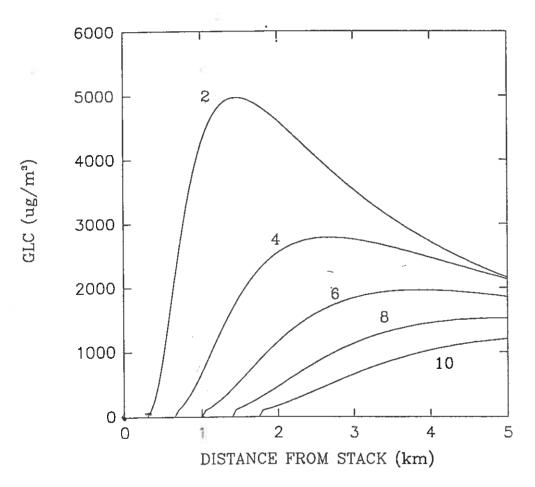
Figure 6 Centreline glc as a function of distance from stack for windspeeds 2,4,6,8, & 10m/s - Base case lead smelter emissions.
